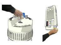
Eliminate any traces of moisture on the filling connectors of the stationary tank and the FREELOX PORTABLE using a **clean**, **lint-free cotton cloth** (moisture leads to the formation of frost on the connector and can cause oxygen leaks).
