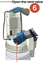
Open the vent valve lever Hold the FREELOX PORTABLE by its top part and push the ejection button.
