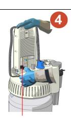
Maintain this pressure using one hand, and with the other hand, open the vent valve lever completely using a moderate amount of pressure.
