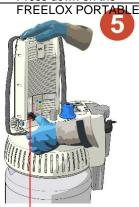
Release the vent valve lever
