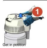
Once the protective cap has been removed from the stationary tank's filling connector, position vourself in front of it. in other words, in front of the condensate collector. in order to protect yourself from the flow of cold oxygen. This will also prevent the oxygen released through the tank's air vents during filling from accumulating in your clothing and posing a potential fire hazard later on.
