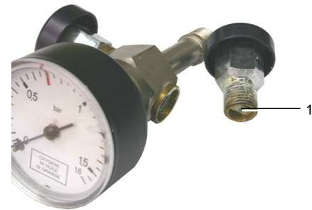
Figure 9-1: Blowing out the valve's seat.
