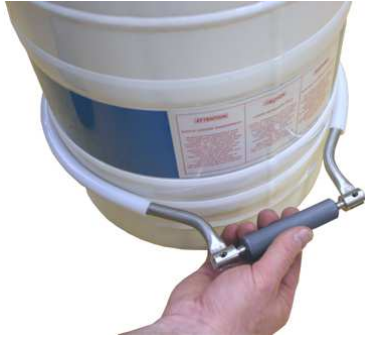
Figure 7-8: removing the pouring handle.
