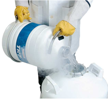
Figure 8-1: filling from a TR vessel; step 1.
