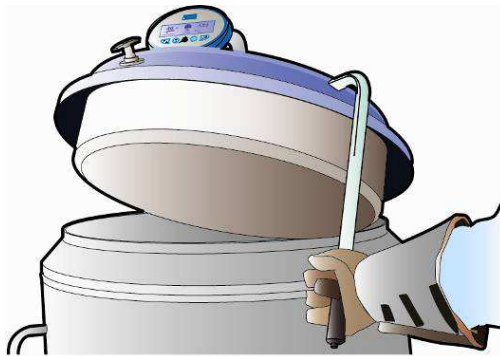
Figure 8-10: Opening or closing the assisted cap - ESPACE 331 and 661
