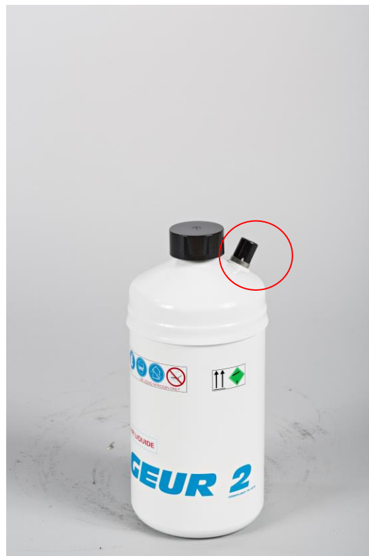
Figure 4-1: Example location of the pump check valve on Voyageur 2
